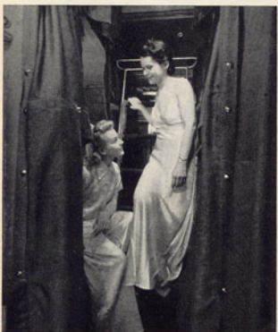
FOR SLEEPING , three tiers of berths, one above the other, are provided. The new rubber mattress is used in each, and each berth has individual curtains and individual air conditioning. Steps to upper berths make it easy to "hit the hay".
