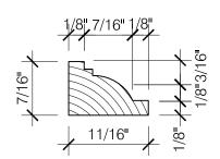
$5 \frac{\text{GLASS STOP DETAIL}}{\text{SCALE: 1'-0"} = 1'-0"}$
