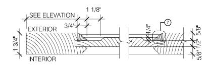
$2\frac{\text{SECTION AT STILE/RAIL AND PANEL}}{\text{SCALE: } 3^{\text{\tiny{II}}} = 1^{\text{\tiny{I}}} \cdot 0^{\text{\tiny{I}}}}$
